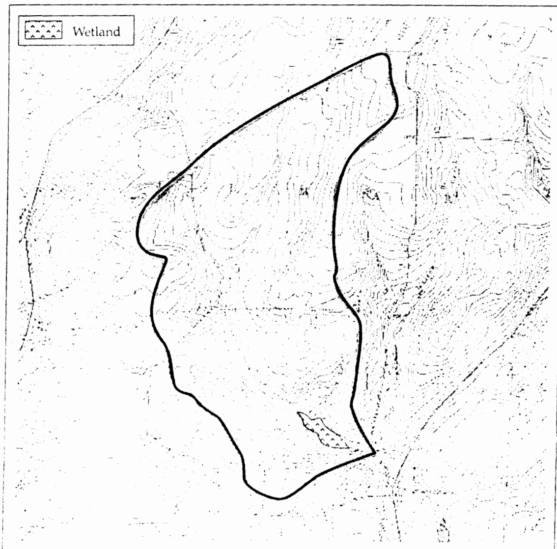
Example of determining the watershed for a wetland on a first order stream.
