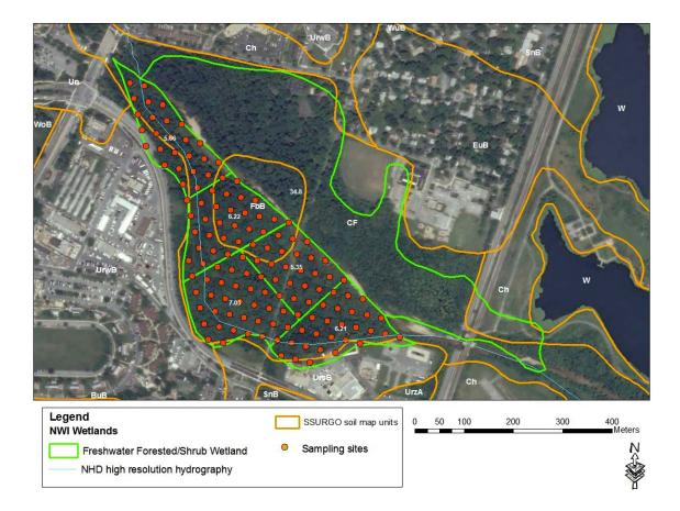
Figure 5. Wetland assessment cells with sampling grid node overlay and acreage shown. The spacing on the grid node can easily be adjusted by the GIS software.
