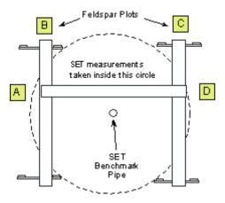
Figure 14. Feldspar plot locations with an SET pipe and permanent platform (from the USGS Surface Elevation Table website at <u>http://www.pwrc.usgs.gov/set/</u>).
