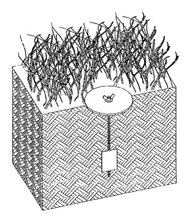
Figure 11. Schematic diagram of plexiglass sedimentation disk (from Kleiss, 1993).
