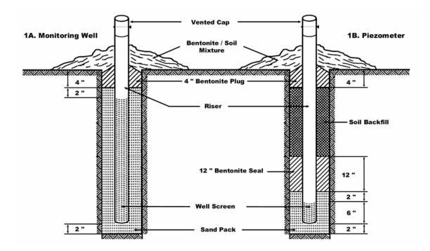
Figure 1. Diagram of installed monitoring well and piezometer. From Sprecher (2000).
