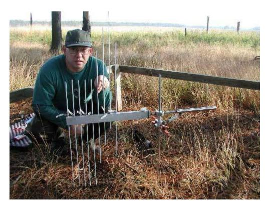
Figure 12. Reading the Rod SET at Blackwater National Wildlife Refuge. (Photo from the USGS Surface Elevation Table website at <u>http://www.pwrc.usgs.gov/set/readSET.html</u>.)
