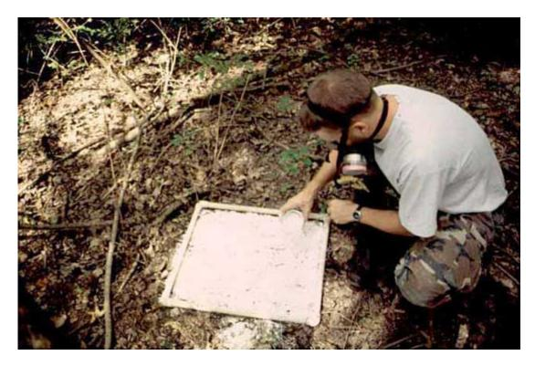
Figure 10. Installing a feldspar marker horizon in a forested wetland (photo is from the USGS Surface Elevation Table website at <u>http://www.pwrc.usgs.gov/set/</u>)
