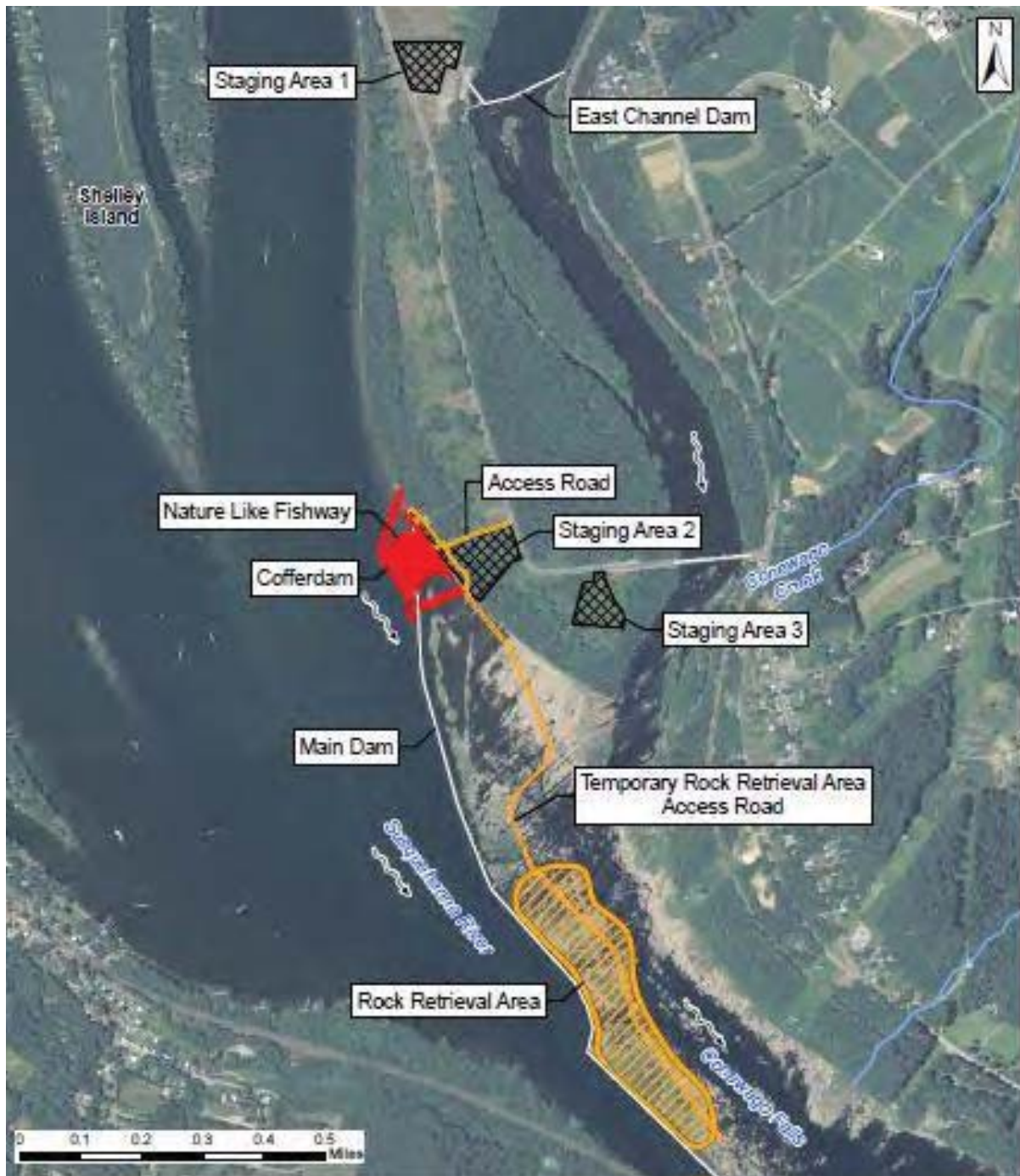
Figure 3-14. Proposed location of the York Haven nature-like fishway and associated construction sites (Source: York Haven Power filing of updated figure for Nature-like Fishway Conceptual Design Final Report, filed June 10, 2013).
