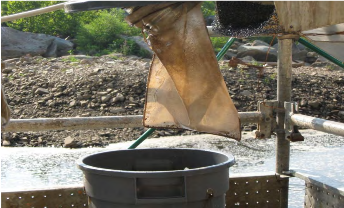
FIGURE 3-10: MESH BAG HOUSED IN PERFORATED TRASH CAN.
