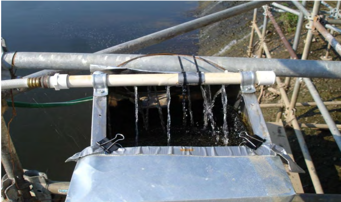
FIGURE 3-8: SPRAY BAR SYSTEM.
