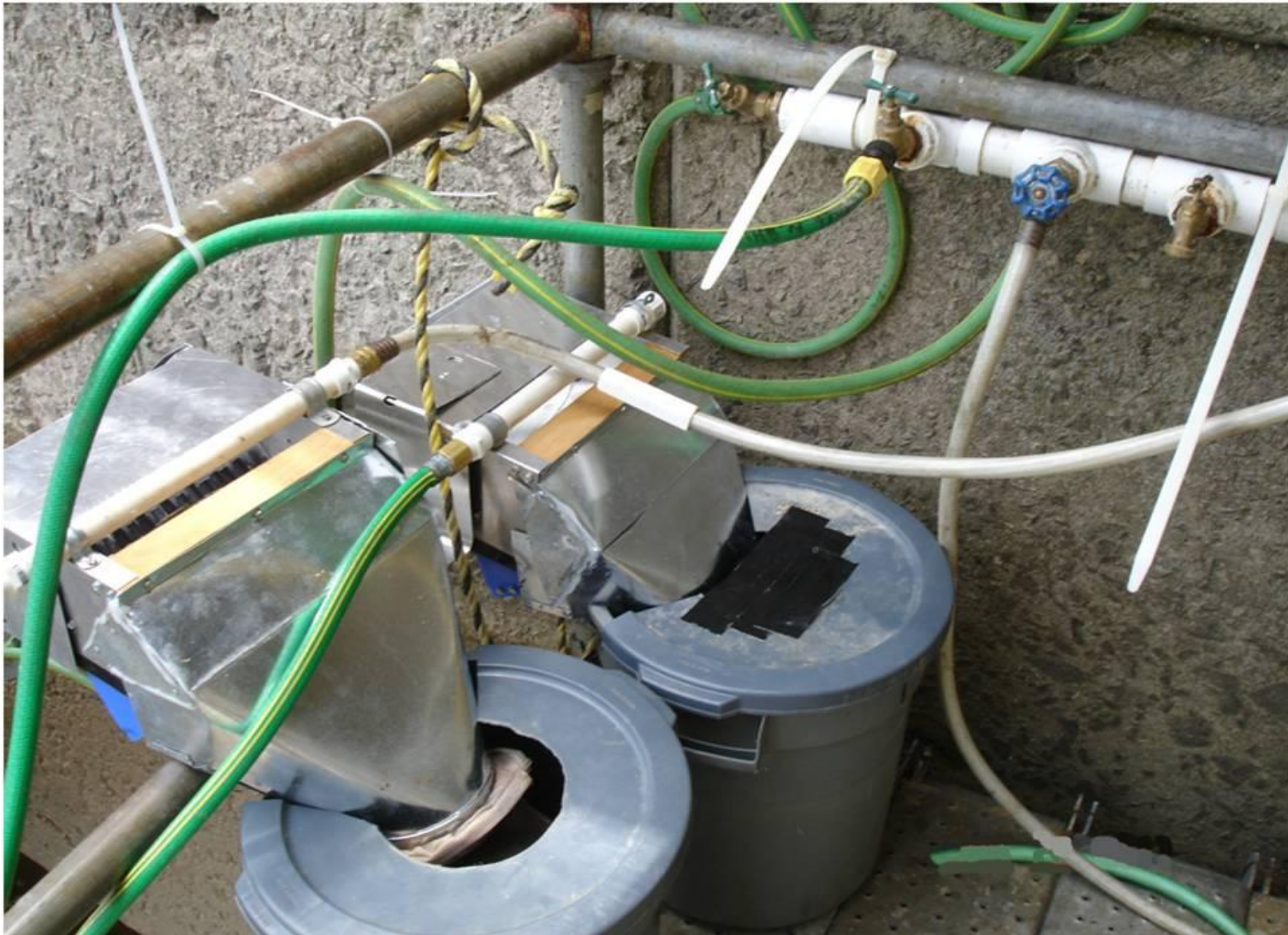
FIGURE 2-8: WATER SUPPLY MANIFOLD, SPRAY BARS, AND HOLDING CONTAINERS.
