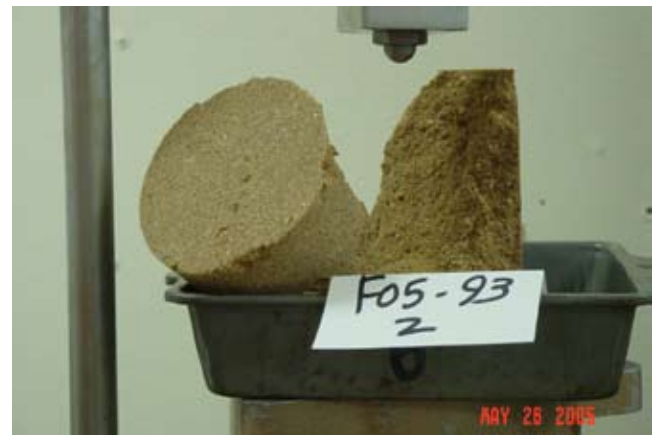
Figure 45B-5 Compressive strength specimen
