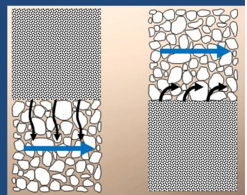
Figure 26-28. Contact Erosion Process (adapted from ICOLD, 2012 Draft)
