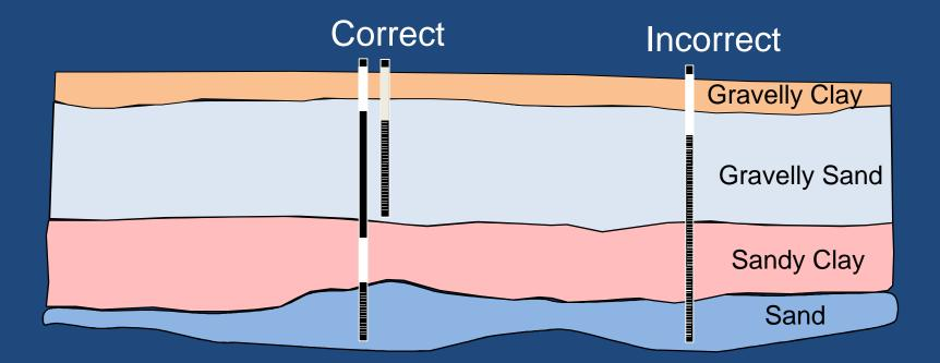
These two piezometers measure pressures in two distinct strata. What pressure does this piezometer measure?
