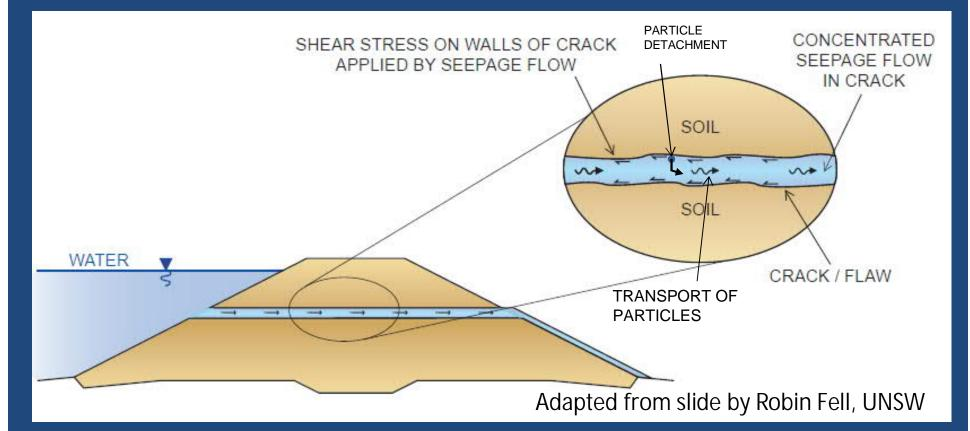
Erosion along sides of an opening (crack). Erosion initiates if hydraulic shear stress > critical shear stress of the soil.
