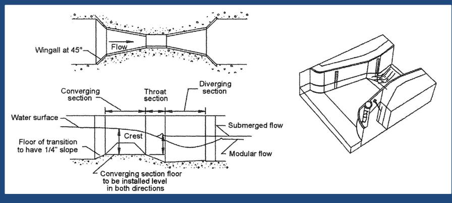
Reference: ASCE, Guidelines for Instrumentation and Measurement for Monitoring Dam Performance, 2000
