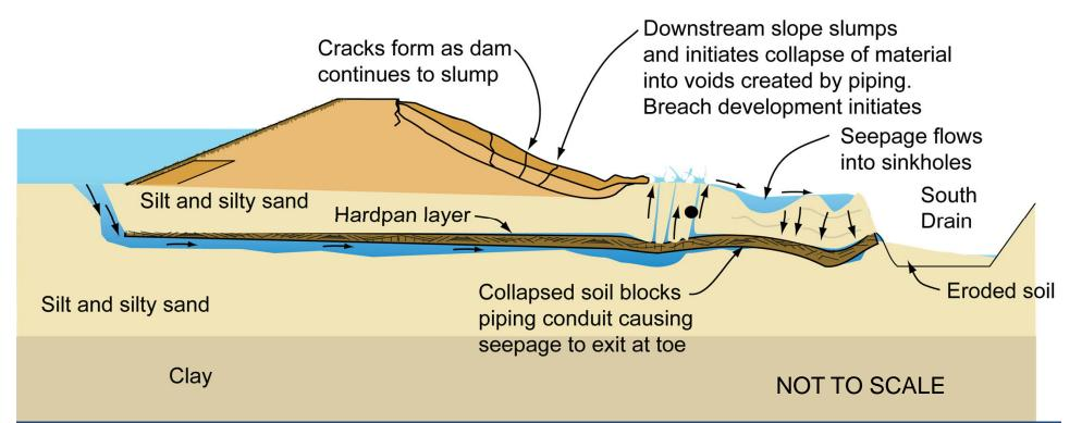
IE Through Foundation (failure in progress)
