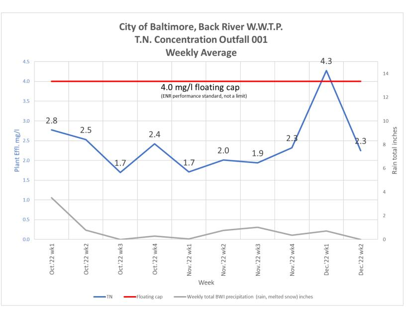
\*Back River WWTP has informed MDE that the high TN results are due to issues with methanol addition and internal recycling pumps. MDE is working with Back River WWTP and MES to ensure these issues do not occur in the future.
