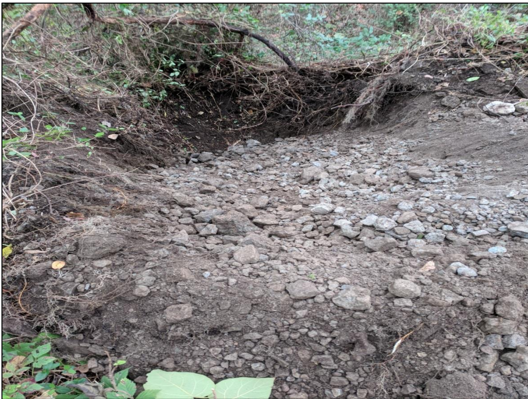
Photo 6: View of A5-003-TP after excavation activities. View is from above looking down the side of the berm. Fine to coarse grained soils (silt, sand, and gravel) and slag fill materials were observed. PID reading of 3.4 ppm was recorded.
