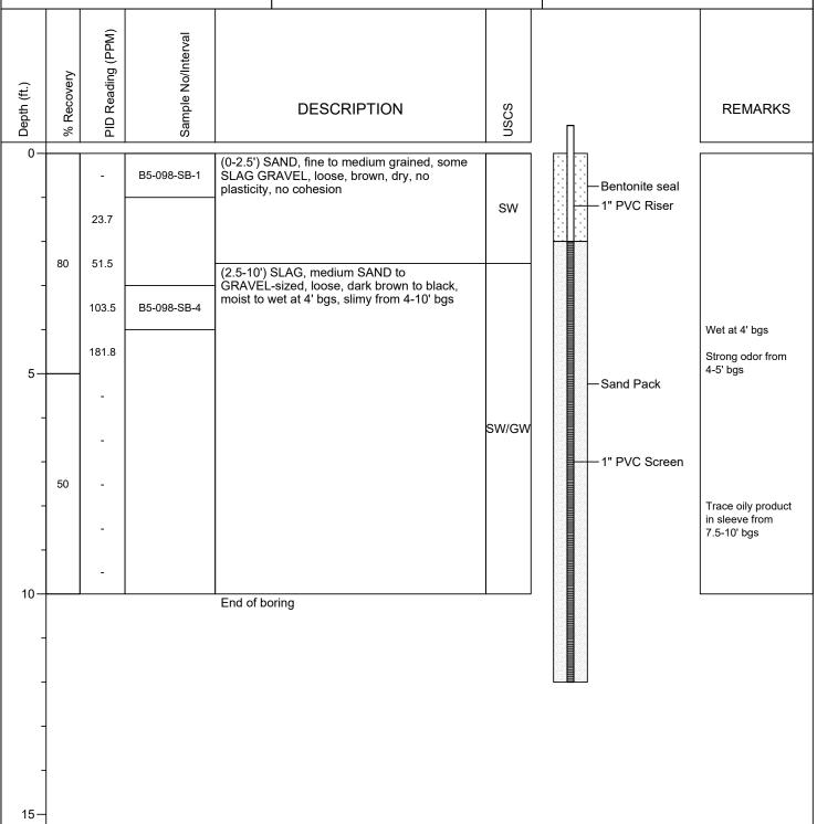
Boring logged to 10' bgs and extended to 12' bgs during piezometer installation.
