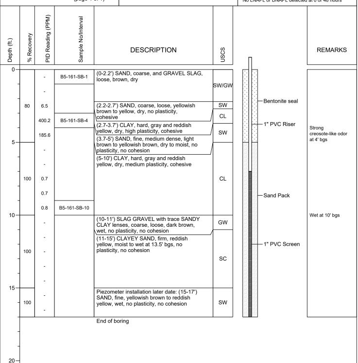
Boring terminated at 17' bgs due to water and piezometer installation.
