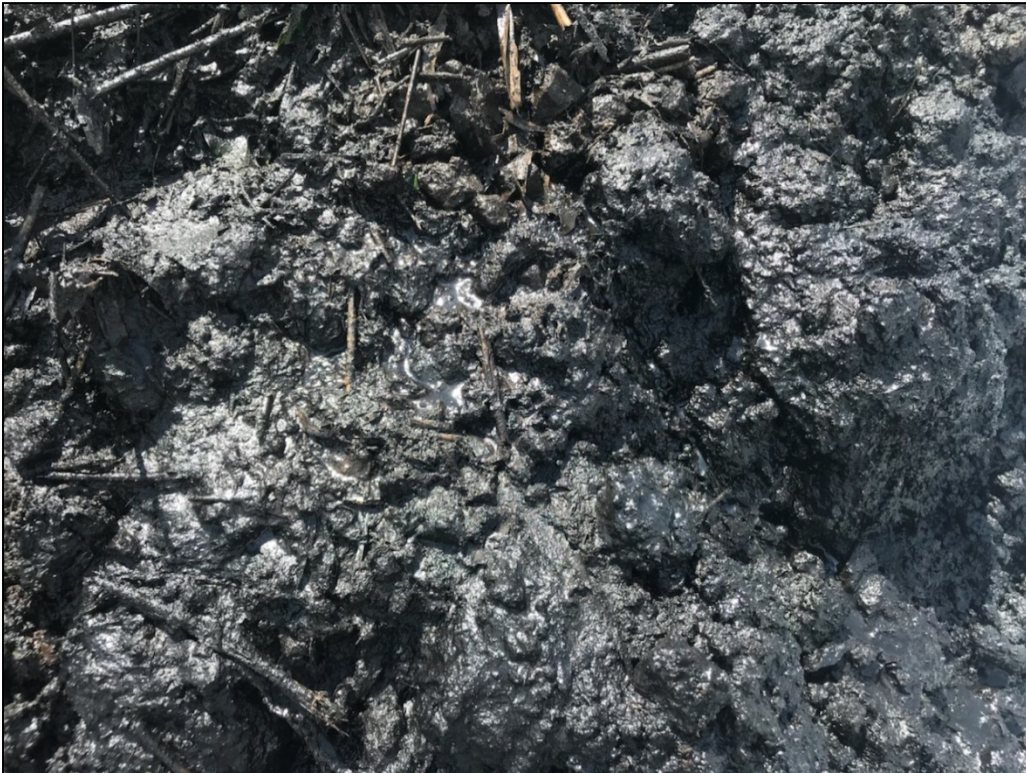
Photo 6: View of excavated material from test pitting activities at the PORI Lagoon.
