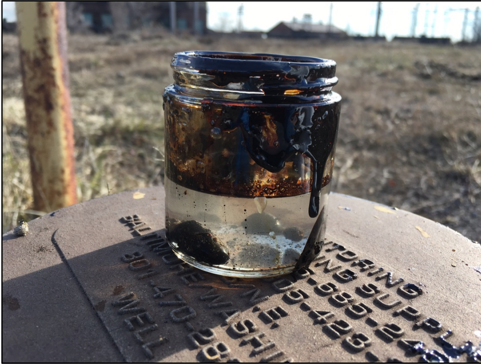
Photo 1: View of NAPL collected from a B18 well. Take note of the NAPL observed as LNAPL and DNAPL.
