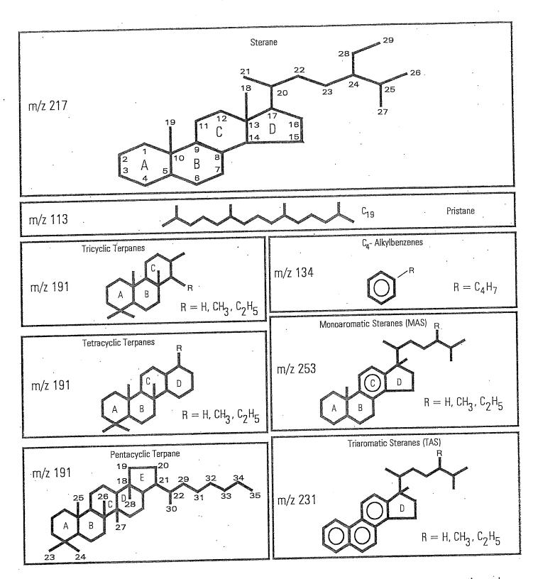
The compound structures of pristane, C<sub>4</sub>-alkylbenzenes, sterane; terpanes; monoaromatic and triaromatic steranes
