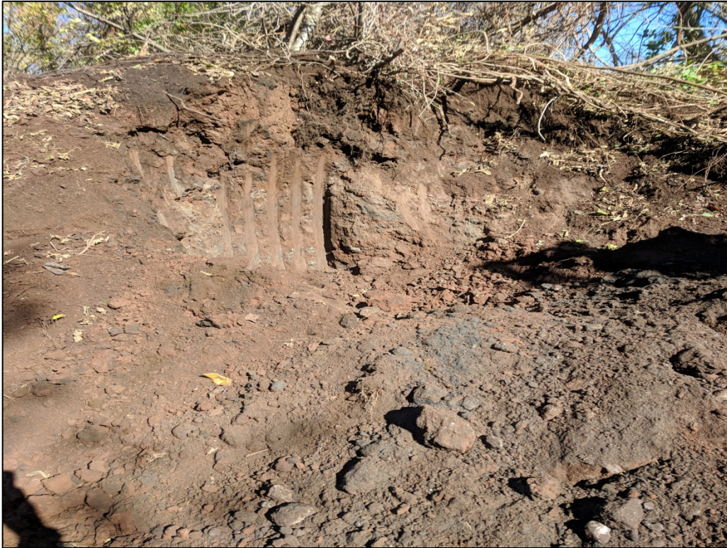
Photo 21: View of test pit at A7-008-TP after excavation. Soils appear to consist of silty clay. No visible contamination is evident and PID reading equals 6.7.
