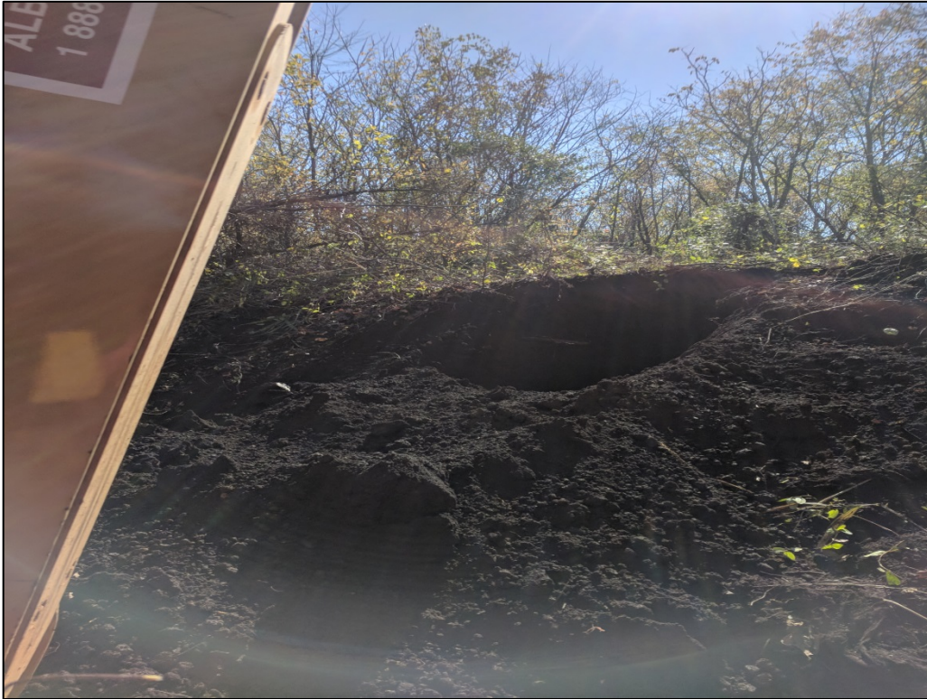
Photo 17: View of test pit at A7-006-TP after excavation. No visible contamination is evident and PID reading equals 7.0.
