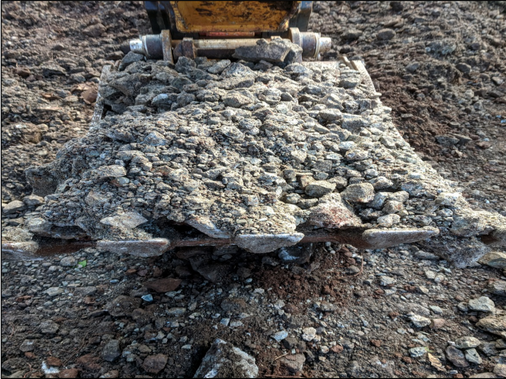
Photo 11: View of the soil observed during test pit activities at A7-004-TP. Soils appear to consist of gravel. No visible contamination is evident.
