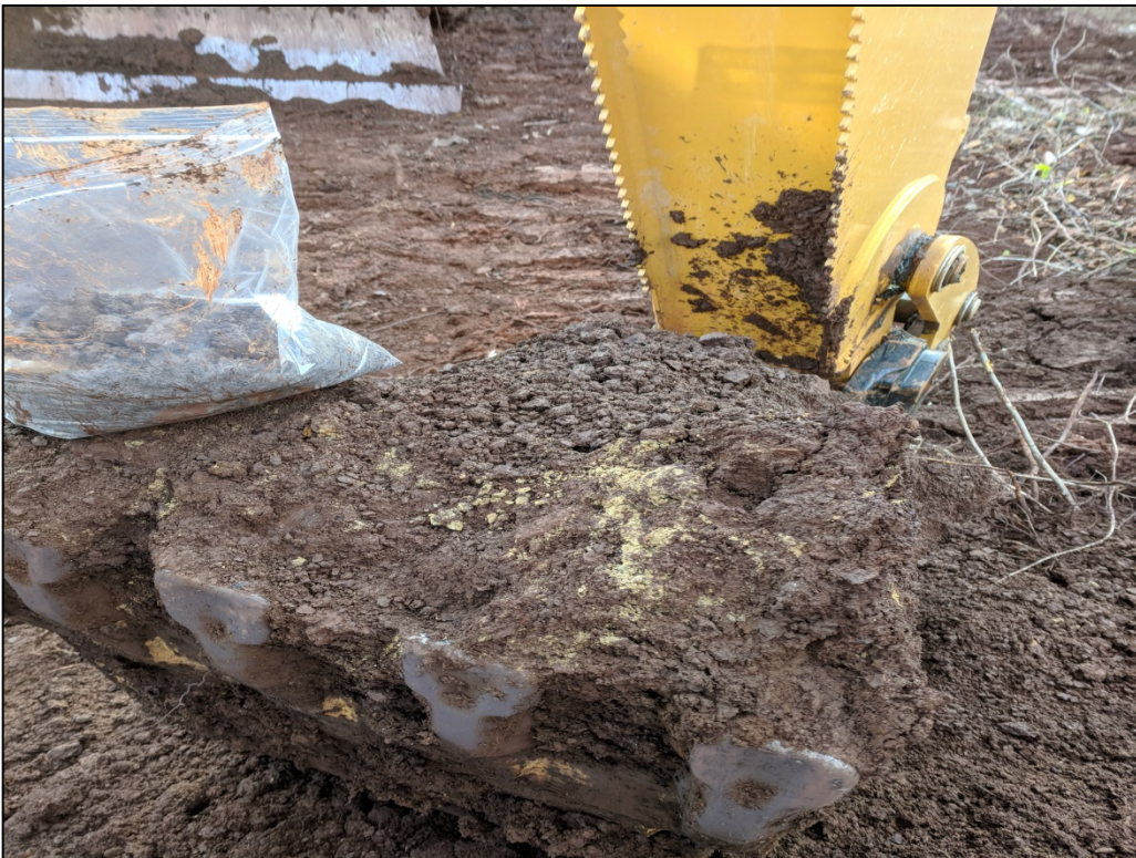
Photo 2: View of the soil observed during test pit activities at A7-001-TP. Soils appear to consist of silty clay. No visible contamination is evident.
