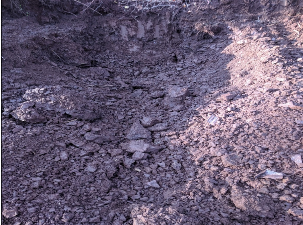
Photo 3: View of test pit at A7-001-TP after excavation. No visible contamination is evident and PID reading equals 3.9.
