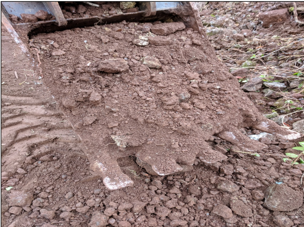
Photo 8: View of the soil observed during test pit activities at A7-003-TP. Soils appear to consist of silty clay with gravel. No visible contamination is evident.
