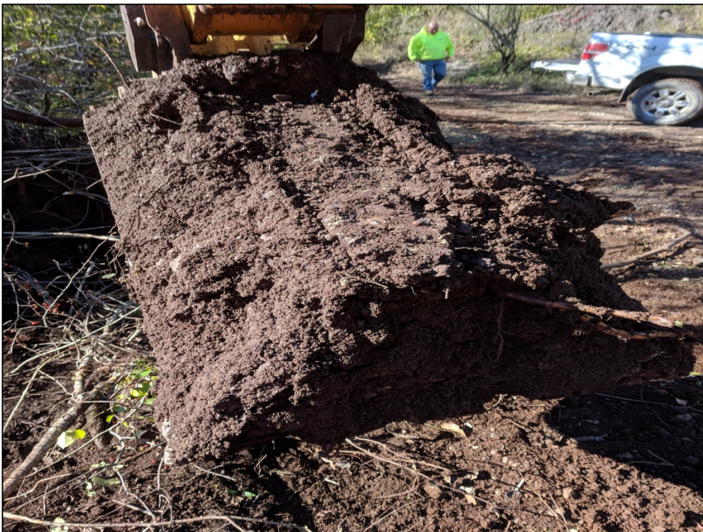
Photo 26: View of the soil observed during test pit activities at A7-010-TP. Soils appear to consist of sandy silt. No visible contamination is evident.
