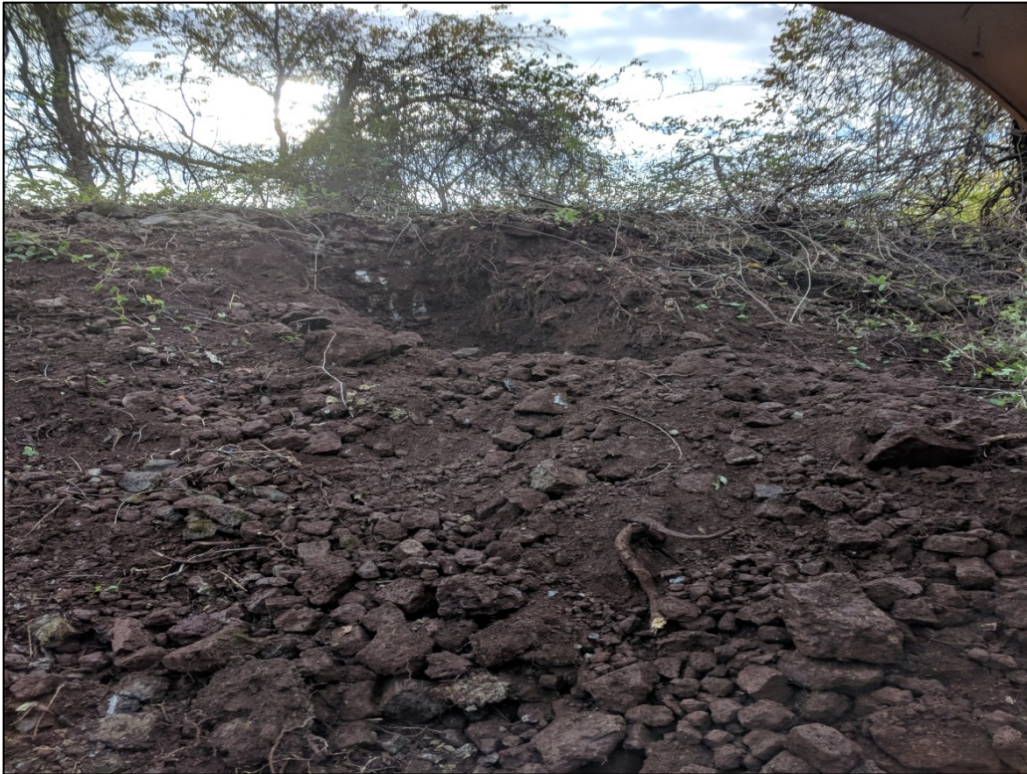
Photo 9: View of test pit at A7-003-TP after excavation. No visible contamination is evident and PID reading equals 2.8.
