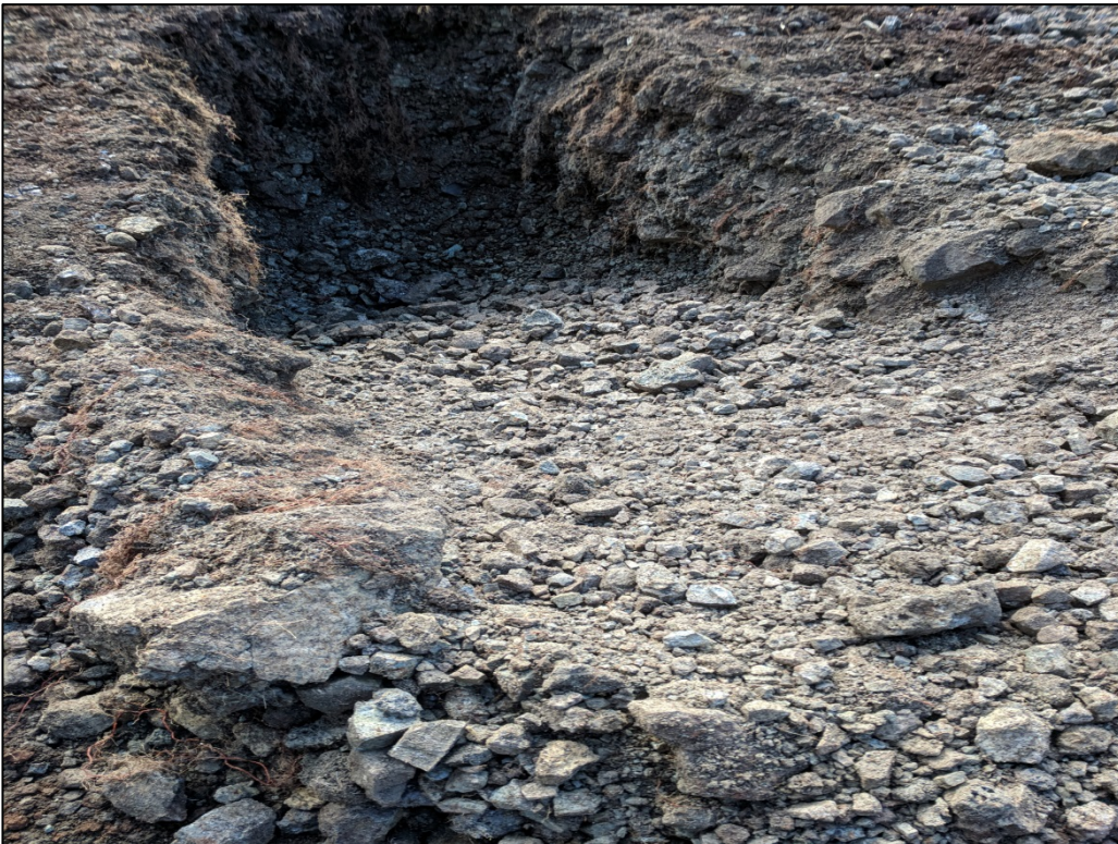
Photo 12: View of test pit at A7-004-TP after excavation. No visible contamination is evident and PID reading equals 2.3.
