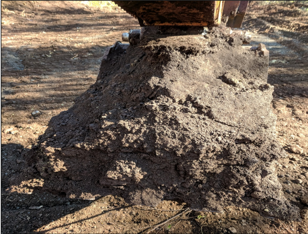
Photo 23: View of the soil observed during test pit activities at A7-009-TP. Soils appear to consist of sandy silty. No visible contamination is evident.
