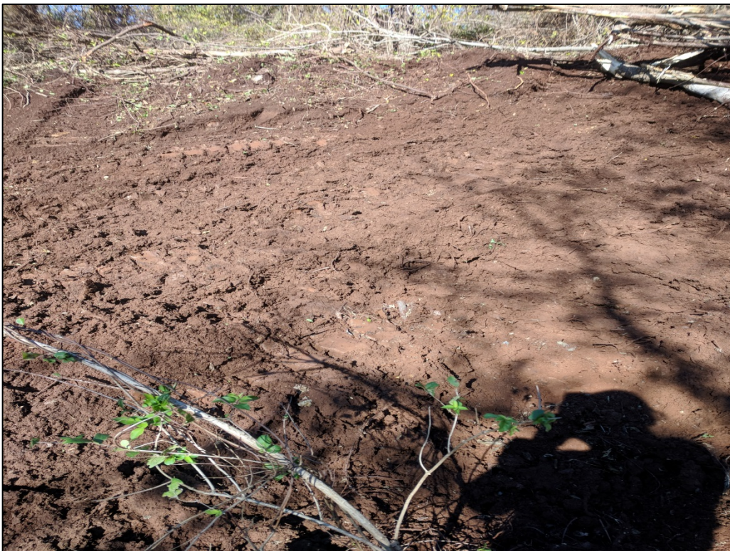
Photo 24: View of test pit at A7-009-TP after excavation. No visible contamination is evident and PID reading equals 3.6.
