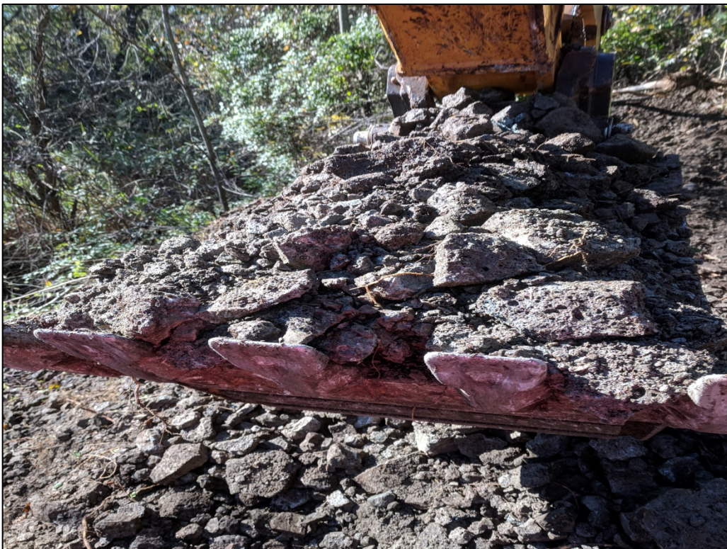
Photo 14: View of test pit at A7-005-TP after excavation. Soils appear to consist of gravel. No visible contamination is evident and PID reading equals 4.6.
