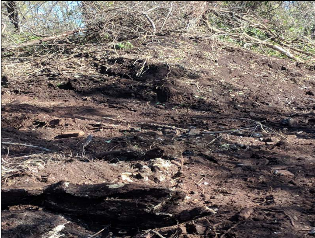
Photo 19: View of test pit at A7-007-TP after excavation. No visible contamination is evident and PID reading equals 7.1.
