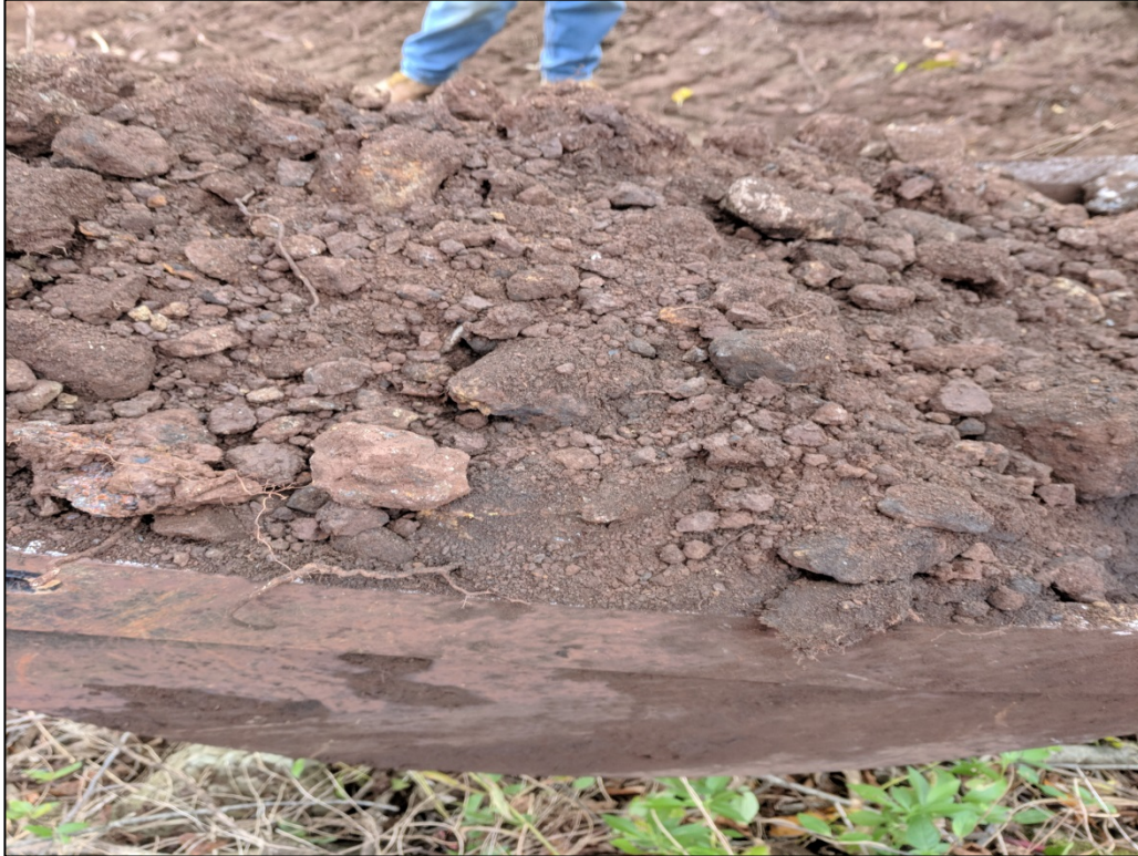
Photo 5: View of the soil observed during test pit activities at A7-002-TP. Soils appear to consist of silty clay with gravel. No visible contamination is evident.
