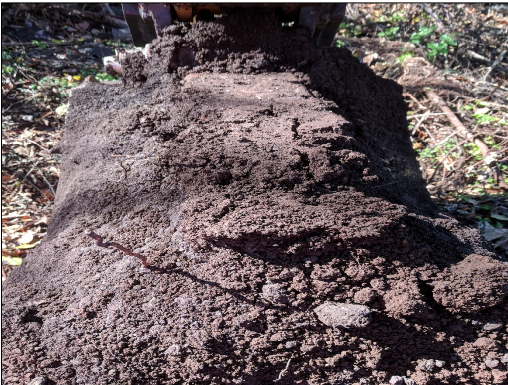
Photo 16: View of the soil observed during test pit activities at A7-006-TP. Soils appear to consist of sandy silt. No visible contamination is evident.
