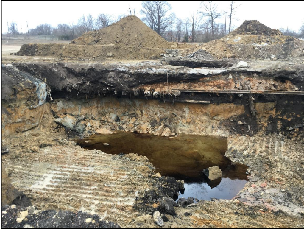
021820-1: Presence of NAPL on the western portion of the eastern test pit excavation area.
