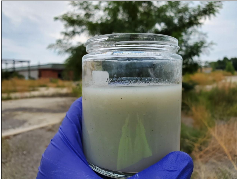
Photograph 1: Unknown product extracted from temporary piezometer A10-006K-PZ. Product is pale gray and moderately thick. Photograph was taken in the field immediately after removal using a bailer.
