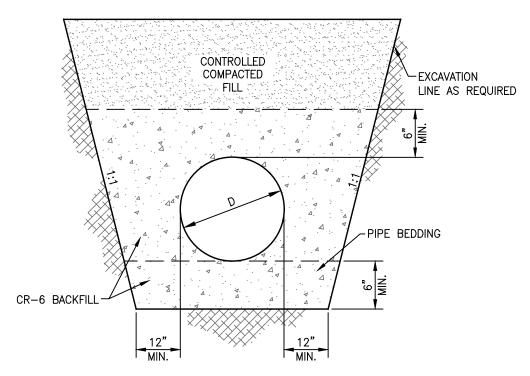
PVC STORM DRAIN PIPE BACKFILL DETAIL NOT TO SCALE
