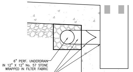
6" X 6" TEE— INSTALL CHECK VALVE DAYLIGHT TO UNDERDRAIN
