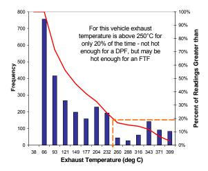
same type of device, unless you operate your equipment in a very different type of duty cycle (i.e., longer periods of idling, lower average engine load). If your make/ model of equipment has never been retrofitted, or if there is any question about its duty cycle, you should collect exhaust temperature data prior to committing to an FTF or passive DPF retrofit.
