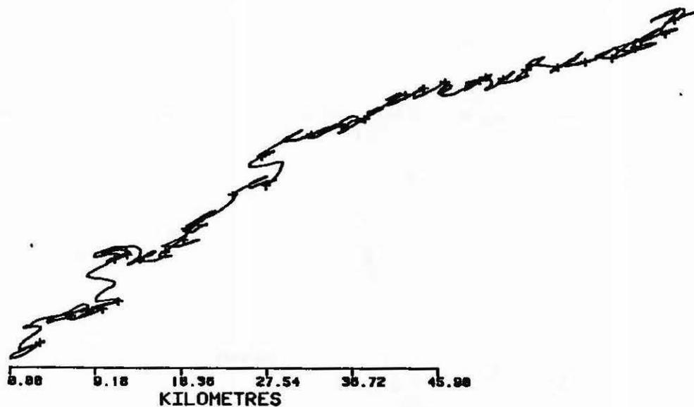
Figure 16. Progressive vector diagram constructed from a current meter record of Station PI in July 1983. 29
