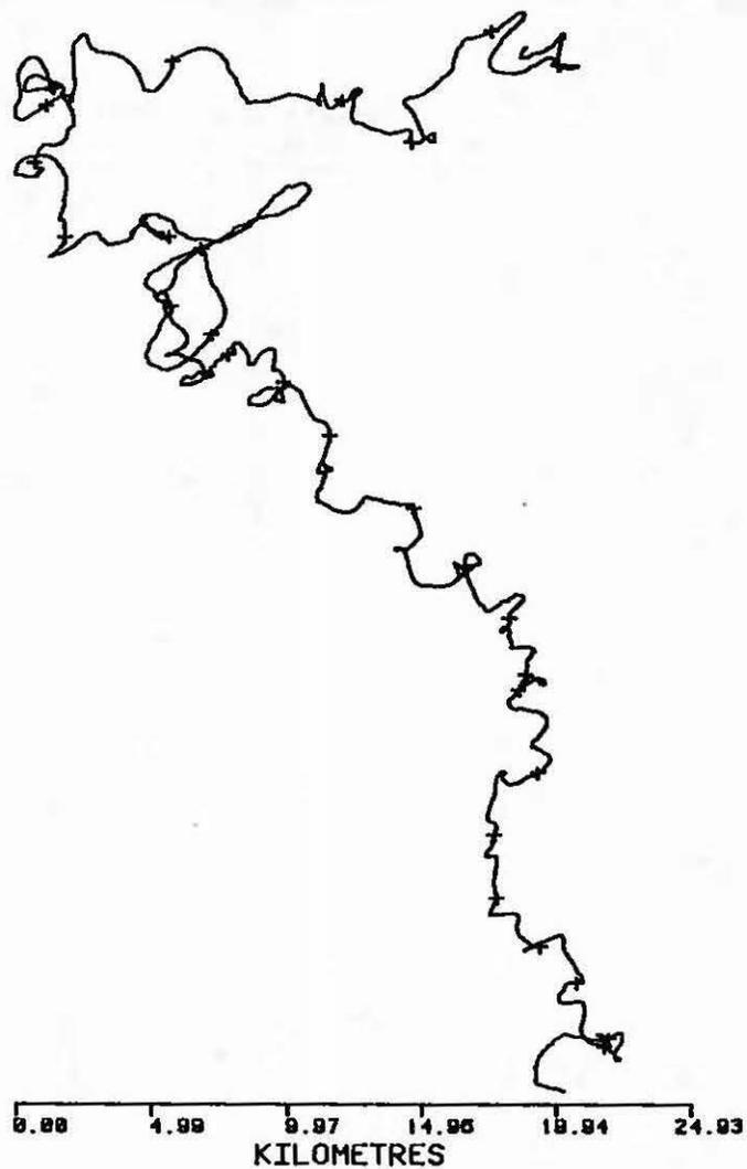
Figure 14. Progressive vector diagram constructed from a current meter record from Station CM3 in July 1983.
