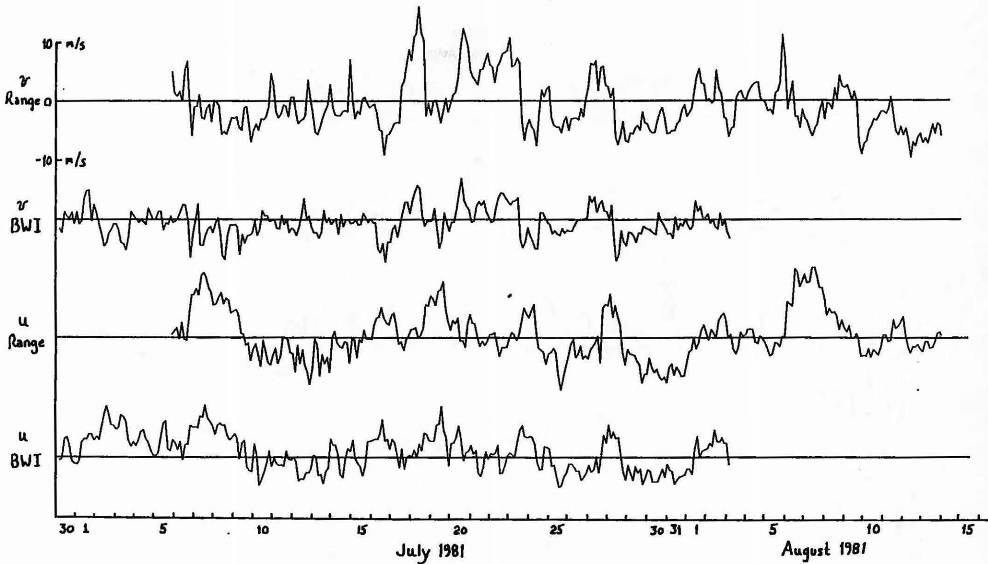
Figure 8. North (v) and east (u) components of wind velocity as measured at Baltimore-Washington International Airport (BWI) and at Craighill Channel Range Light (Range).
