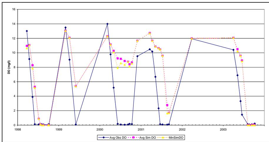
**Figure 13: Observed and Simulated Average Bottom DO Concentrations, Station TR1, All-Forest Scenario, Triadelphia Reservoir**
