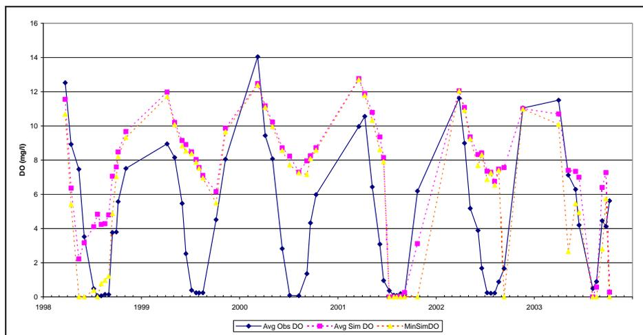
**Figure 14: Observed and Simulated Average Bottom DO Concentrations, Station RG1, All-Forest Scenario, Rocky Gorge Reservoir**
