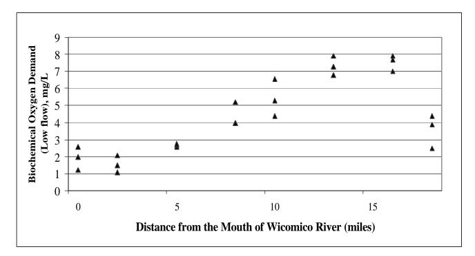
Figure A2: Longitudinal Profile of BOD Data
