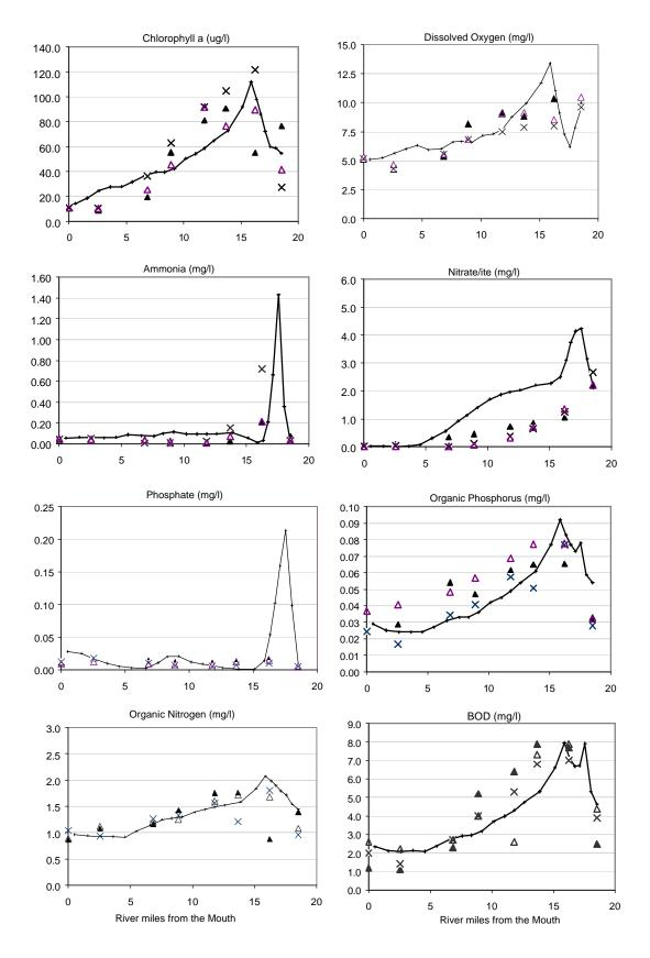
Figure A11: Low Flow Calibration of the Lower Wicomico River Model
