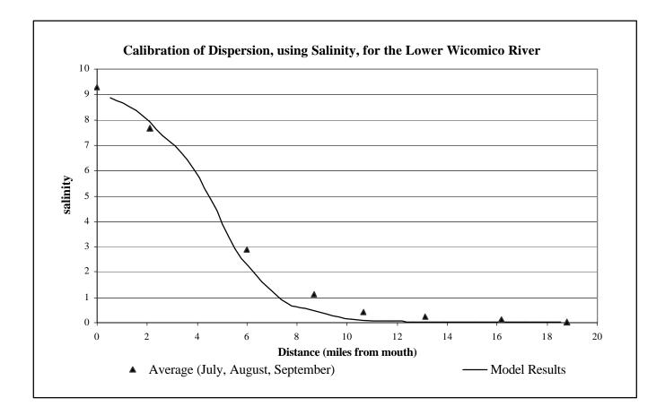
**Figure A8: Results of the Calibration of Dispersion Coefficients for Low Flow**
