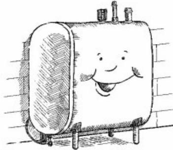
*If you remove a tank from service, be sure to remove fill and vent pipes immediately to prevent a fuel delivery to a location without an attached tank.*
