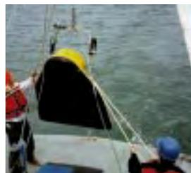
**Use different tow vehicles for desired penetration and resolution. The topside portion remains the same. The FM pulse is user selected based on the sub-bottom conditions at the survey site and the type of sub-bottom features that need to be imaged.**
