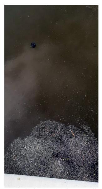
Scum and black solid particles in the final effluent 3/22/22
