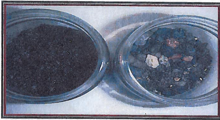
Photograph 2-1: Pre-post Ivey-sol ® Remediation of Refinery Soils
