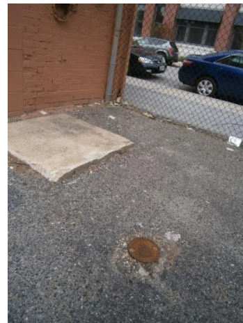
Photograph 6. Groundwater monitoring well in southwestern portion of Furst Brothers
