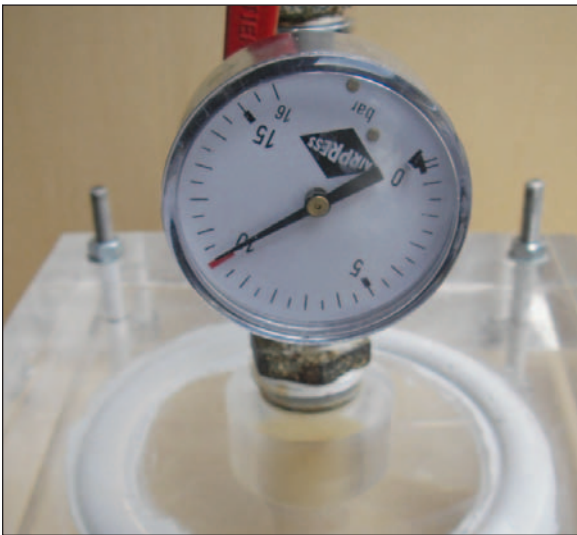
Withstands head pressures in excess of 330 ft.
