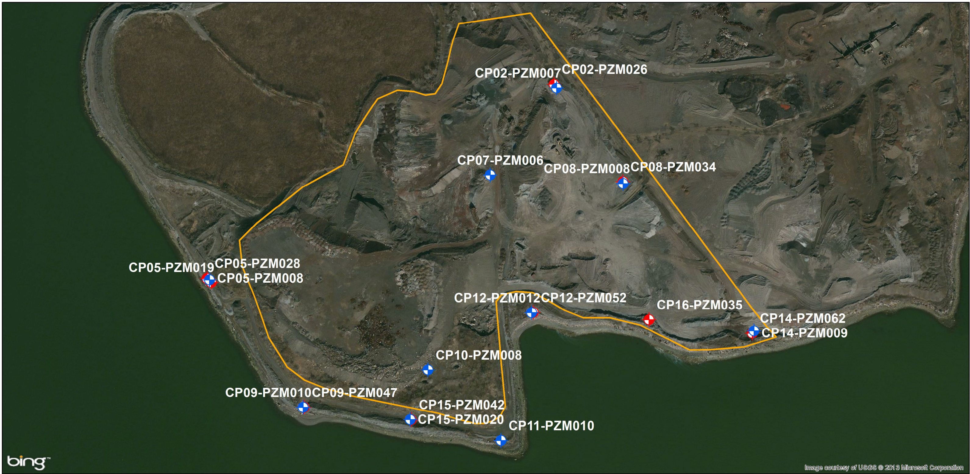
Coke Point Landfill Monitoring Well Locations
