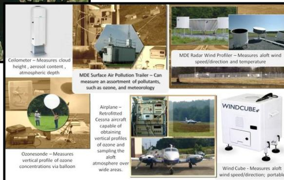
Ceilmeter – Measures cloud height, aerosol content, atmospheric depth
