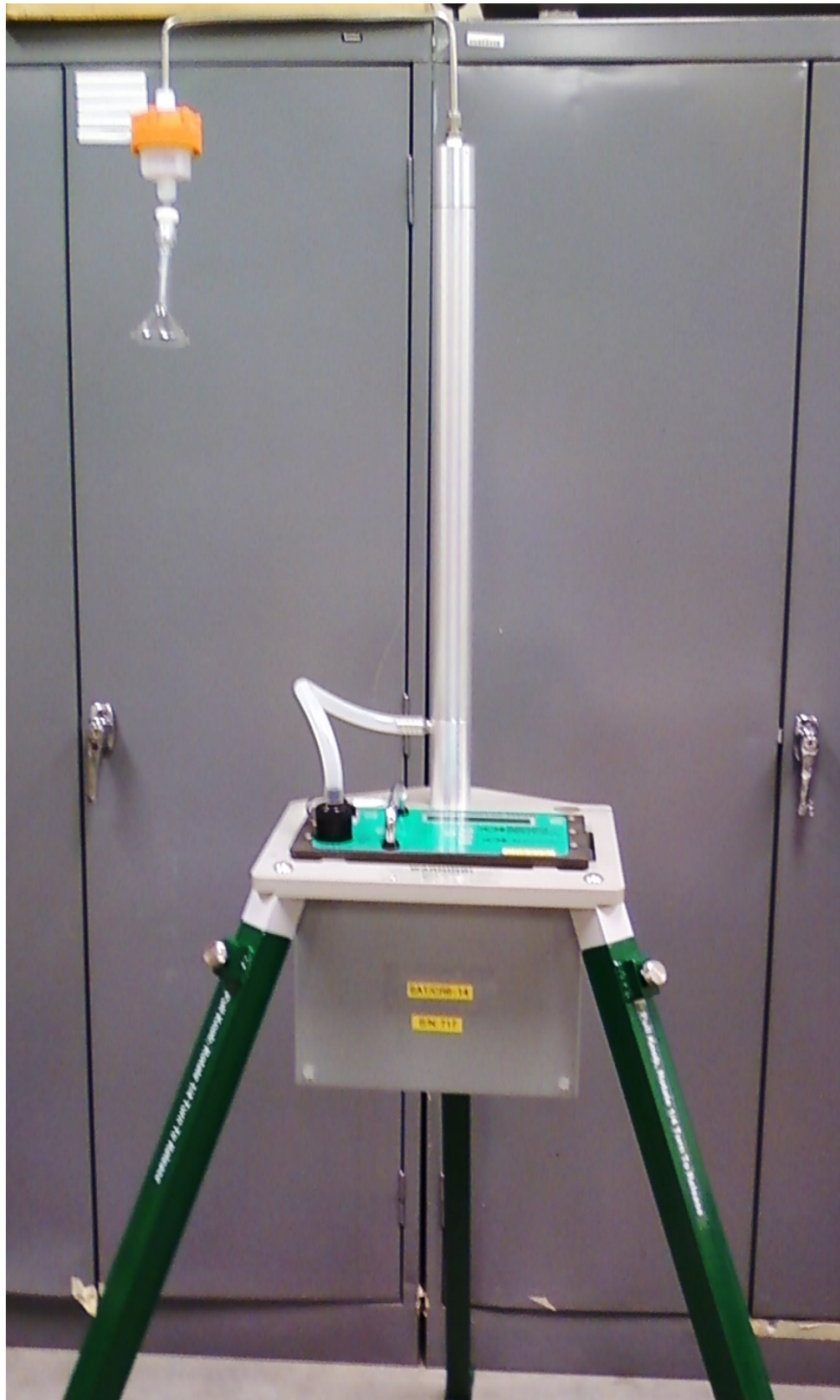
Figure 5-5. PQ100 Assembly with ERG Retrofit
