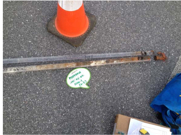
Photo 2: View of soil core collected from boring GTA-1.
