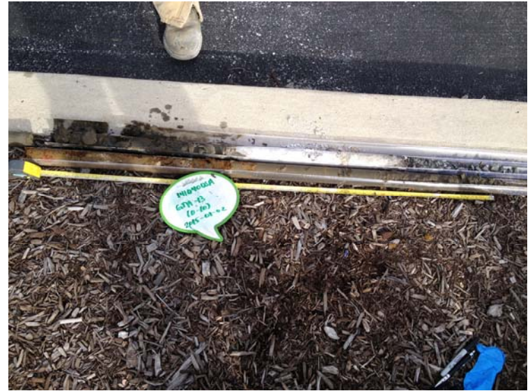
Photo 6: View of soil core collected from boring GTA-13.
