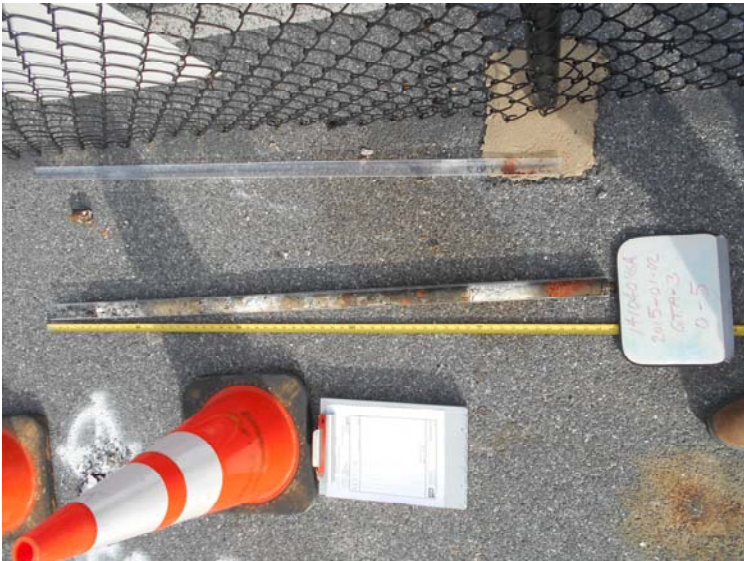
Photo 3: View of soil core collected from boring GTA-3.
