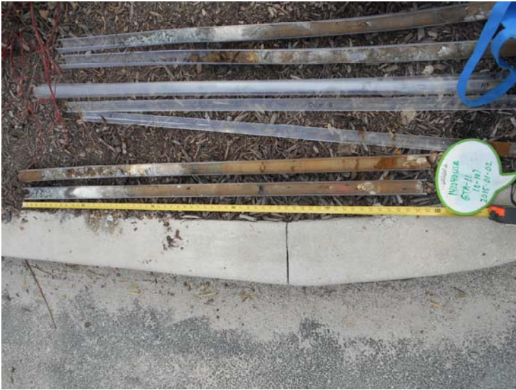
Photo 5: View of soil core collected from boring GTA-11.
