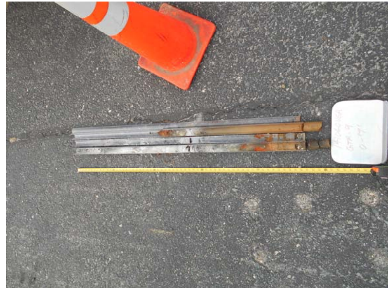
Photo 4: View of soil core collected from boring GTA-9.
