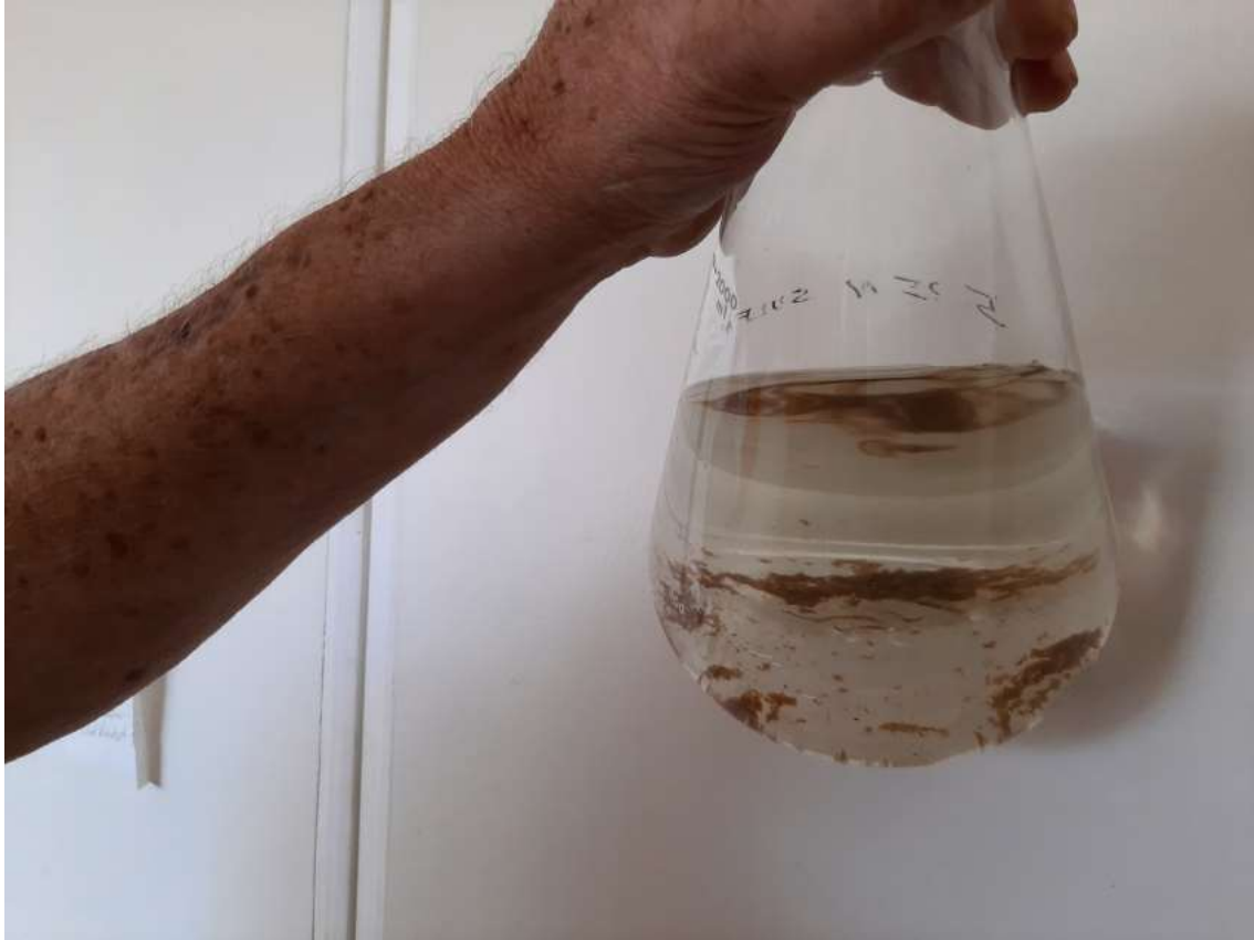
8/16/22 Sample of influent with high amount of suspended solids entering the DNF system at approximately 3:00 a.m.
